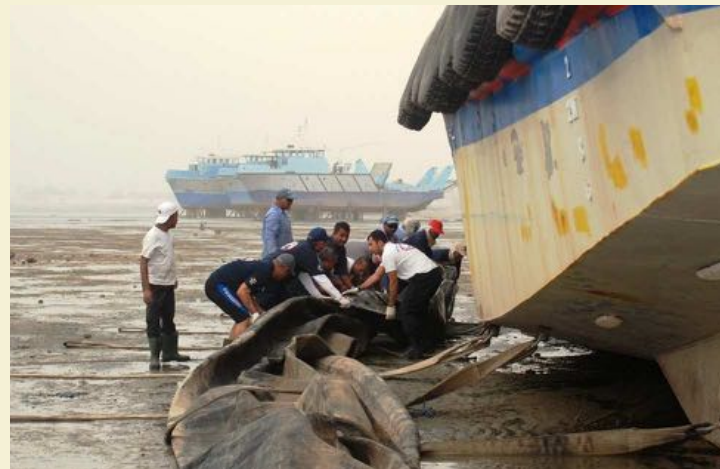
Lift bags, vital to underwater salvage, weigh a great deal themselves and take skills - including teamwork - to get in position during operations.
